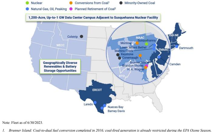
Brunner Island: Coal-to-dual fuel conversion completed in 2016; coal-fired generation is already restricted during the EPA Ozone Season, which is May 1 to September 30 of each year and will cease by year-end 2028. Montour: Coal-to-gas conversion completed in August 2023. Wagner unit 3: Conversion from coal to oil to be complete by year-end 2023.
